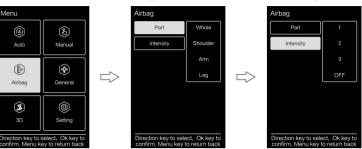
Part: airbags are available for whole body, shoulders, legs and arms. Intensity: it can be chosen from level 1-3. If it it shut down, the pressure should be re-chosen again to adjust the strength.
